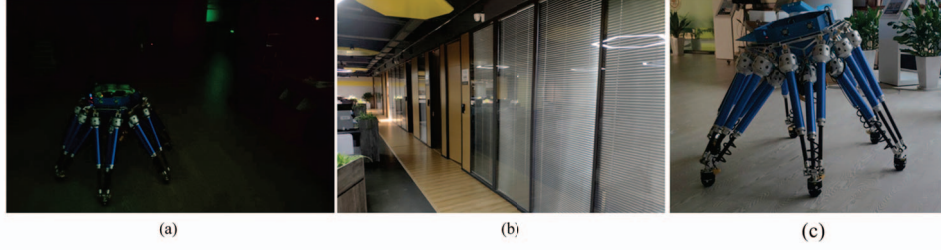
Fig. 3. Experiment Scenes. (a) Small scene odometry estimation in dark environment. Visual odometry is not available when the robot is in the dark environment, but our method can also work well in this scene. (b) Large scene odometry estimation with repeated textures. Visual odometry is not available when the textures in the scene are repeated, but our method does not have this limit. (c) Posture estimation when standing. When the robot stands on the ground, it rotates its body and utilizes 6-DOF force sensors and IMU to estimate posture changes.
